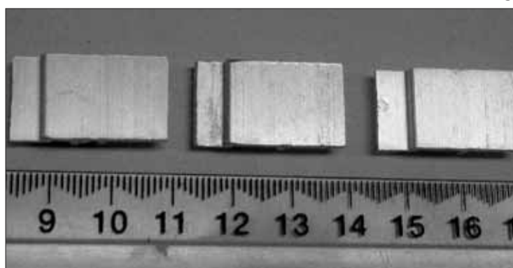
Fig 6 Etched extrusion samples. Left: 40C/5 min; middle: 70C/5 min; right: 90C/5 min. The arrow indicates a streaking defect.
