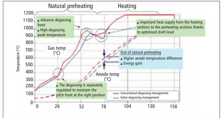
Fig 6 Comparison of heating curves to the new methodology
