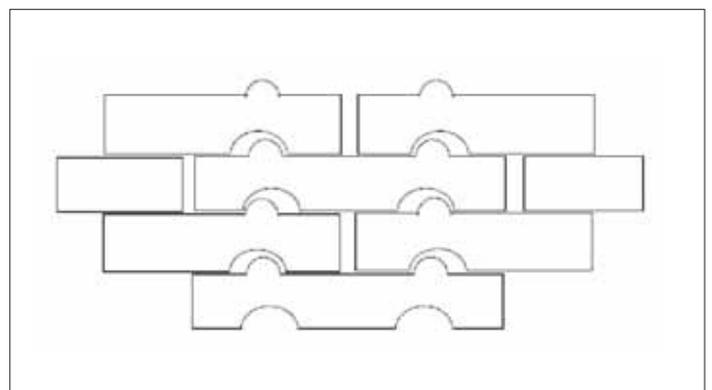
Fig 2 Headwall expansion joint design concept
