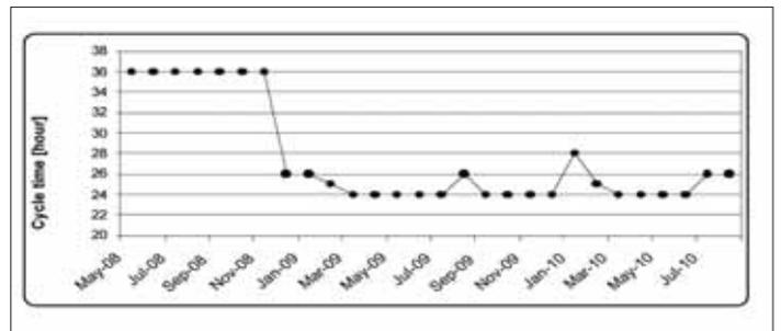
Fig10 Firing cycle evolution
