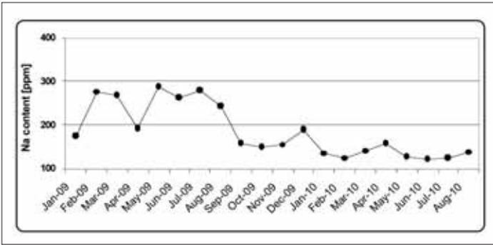
Fig 12 Sodium content in baked anodes
