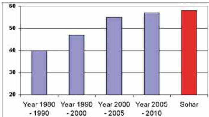
Fig 1 Ratio anode weight/refractory and insulation weight
