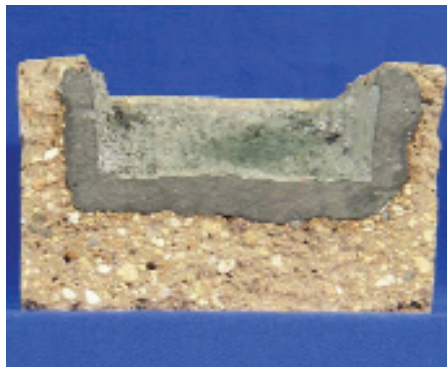
Fig 8 Sub-heat Gunning material tested by method 2
