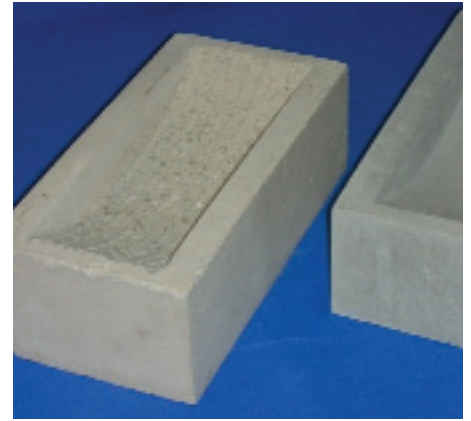
Fig 4 Samples prepared by method 1 (left) and method 2 – as fired (right) and after surface roughing (middle)
