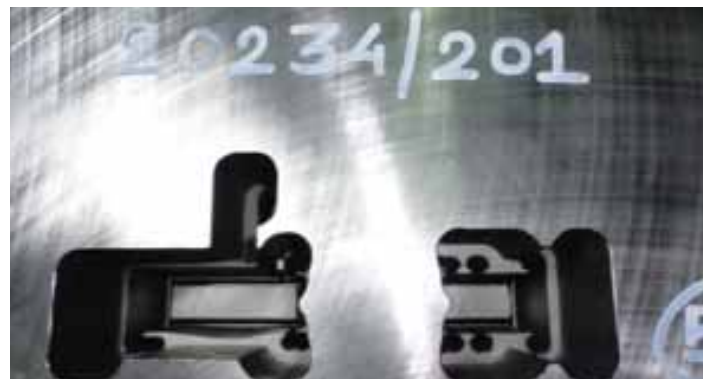
Fig 8. Incorrect layout of Die Cavities
