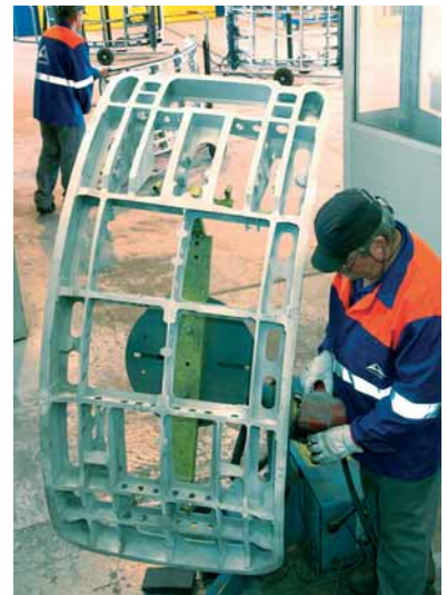
Casting and forging are also researched at Voreppe. A precision cast door for the Dassault Falcon
