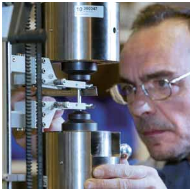
Fatigue tests can be performed on full scale sections in a 2500kN testing rig
