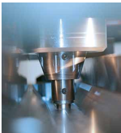
Friction stir welding can reduce machining by joining plate of different thickness
