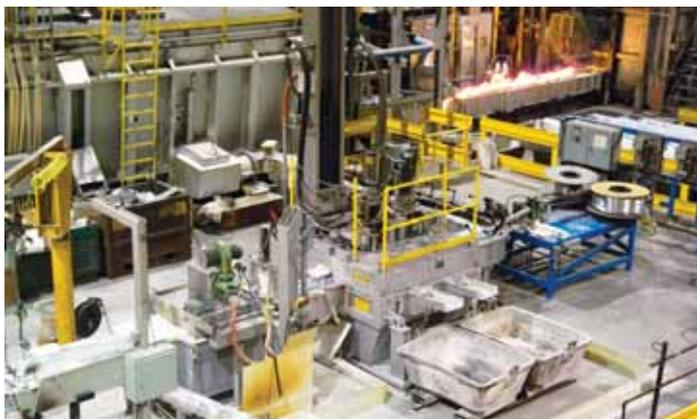
The expanded casthouse at Cressona includes a tilting furnace with pouring trough and SNIF filtration equipment
