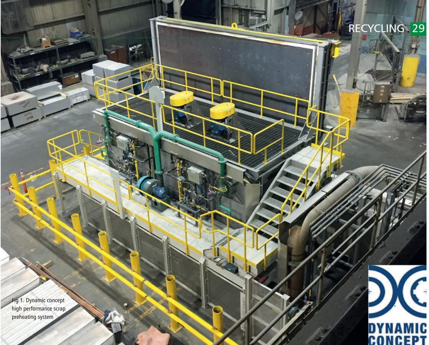
Fig 1. Dynamic concept high performance scrap preheating system
