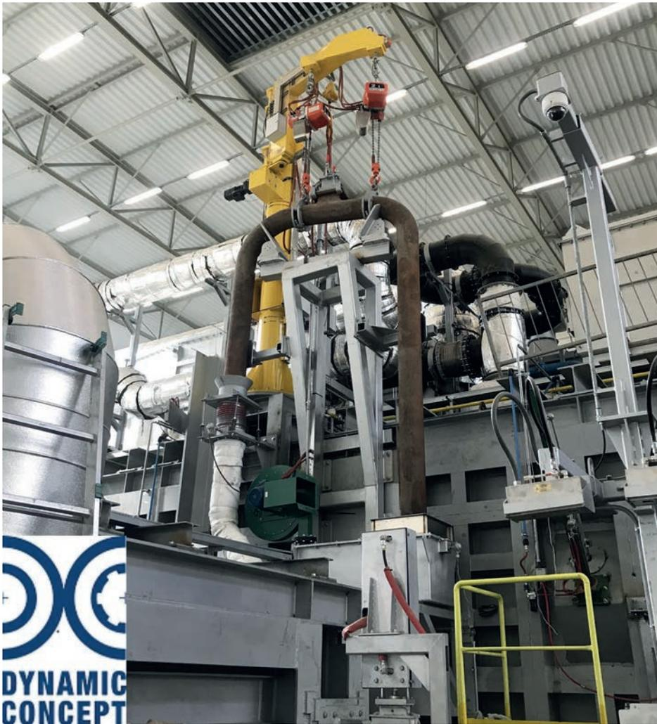
Fig 2. Dynamic concept furnace to furnace metal transfer siphoning system
