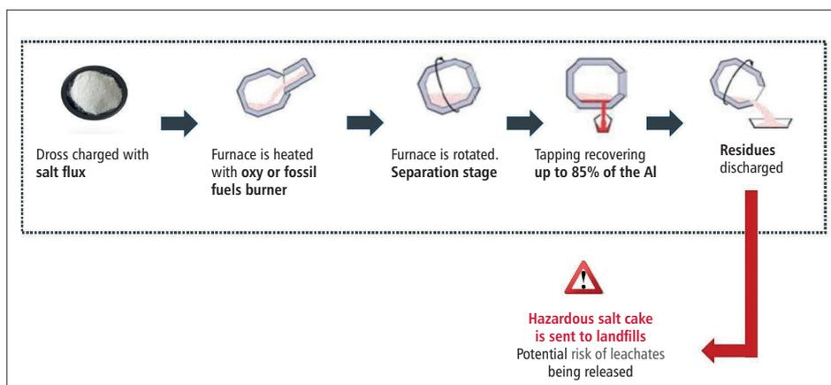
Figure 2. Rotary salt furnace process
