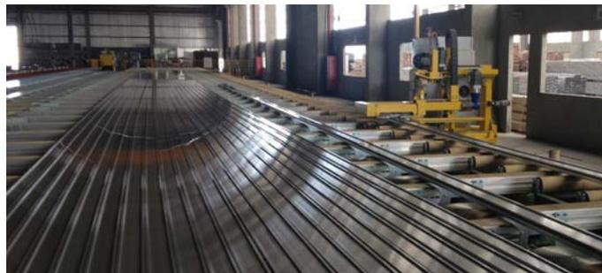
*Single Puller Lateral Type (complete electric)*
