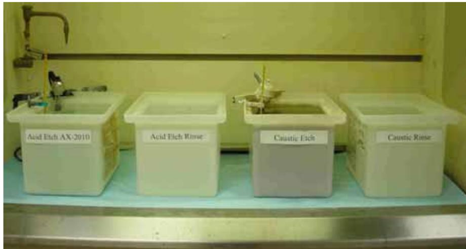
**Figure 2. Houghton Metal Finishing, 20-L Pilot Line**
