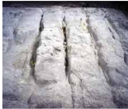
Fig 4 The result of exposing a cleaned cathode surface to air. a) Alumina powder formed by reaction between aluminium carbide and moist air. The ridges are reaction products being pushed up from the narrow joints. b) A view of the destroyed cathode surface after most of the powder has been removed
