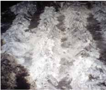
Fig 4 The result of exposing a cleaned cathode surface to air. a) Alumina powder formed by reaction between aluminium carbide and moist air. The ridges are reaction products being pushed up from the narrow joints. b) A view of the destroyed cathode surface after most of the powder has been removed
