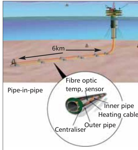
Fig 8 Subsea pipeline configuration reproduced with permission of Technip UK
