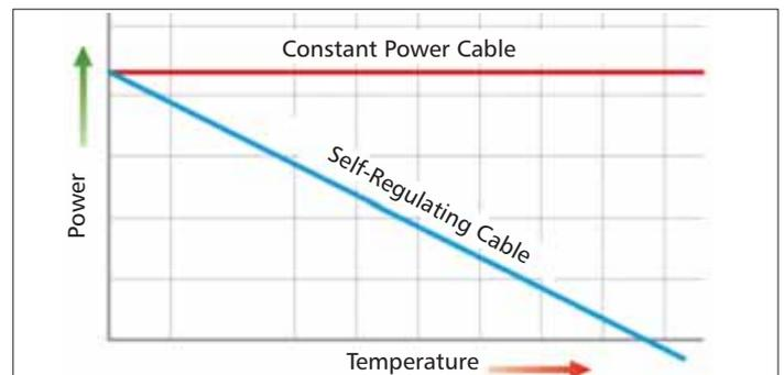
Fig 2 Comparison of power outputs of self-regulating and constant power heaters
