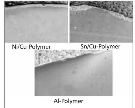
Fig 5 Scanning electron micrographs of metal-polymer interfaces
