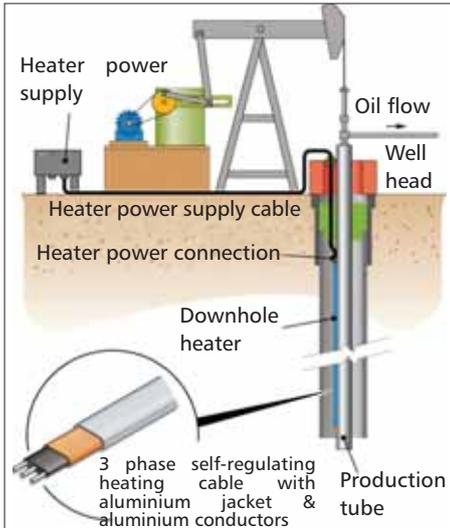
Fig 7 Aluminium 3-phase trace self-regulating
