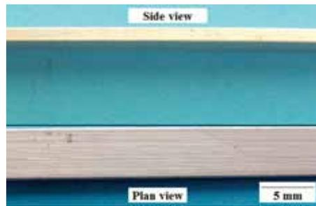
Fig 4 Sample of extruded aluminium conductor
