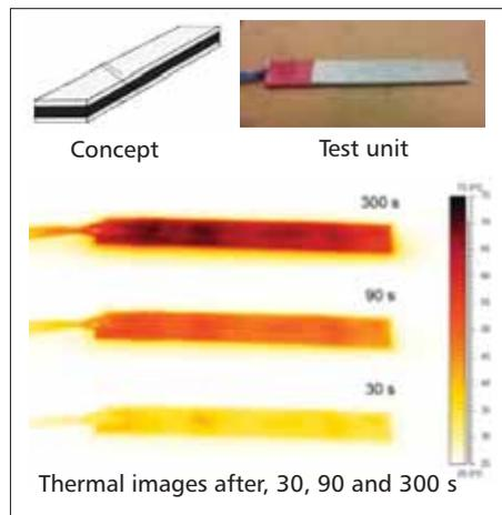
Fig 6 Aluminium laminate heater
