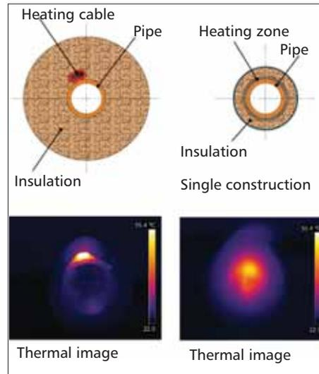
Fig 10 Comparison of trace heating (TH) and aluminium based heated pipe (ABHP)
