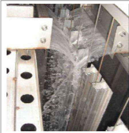
Fig 7 Gardobond® X 4707 for the passivation of aluminum sections in a vertical plant.
