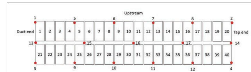
Fig 7. Placement of thermocouple on the cathode for detailed preheating follow-up
