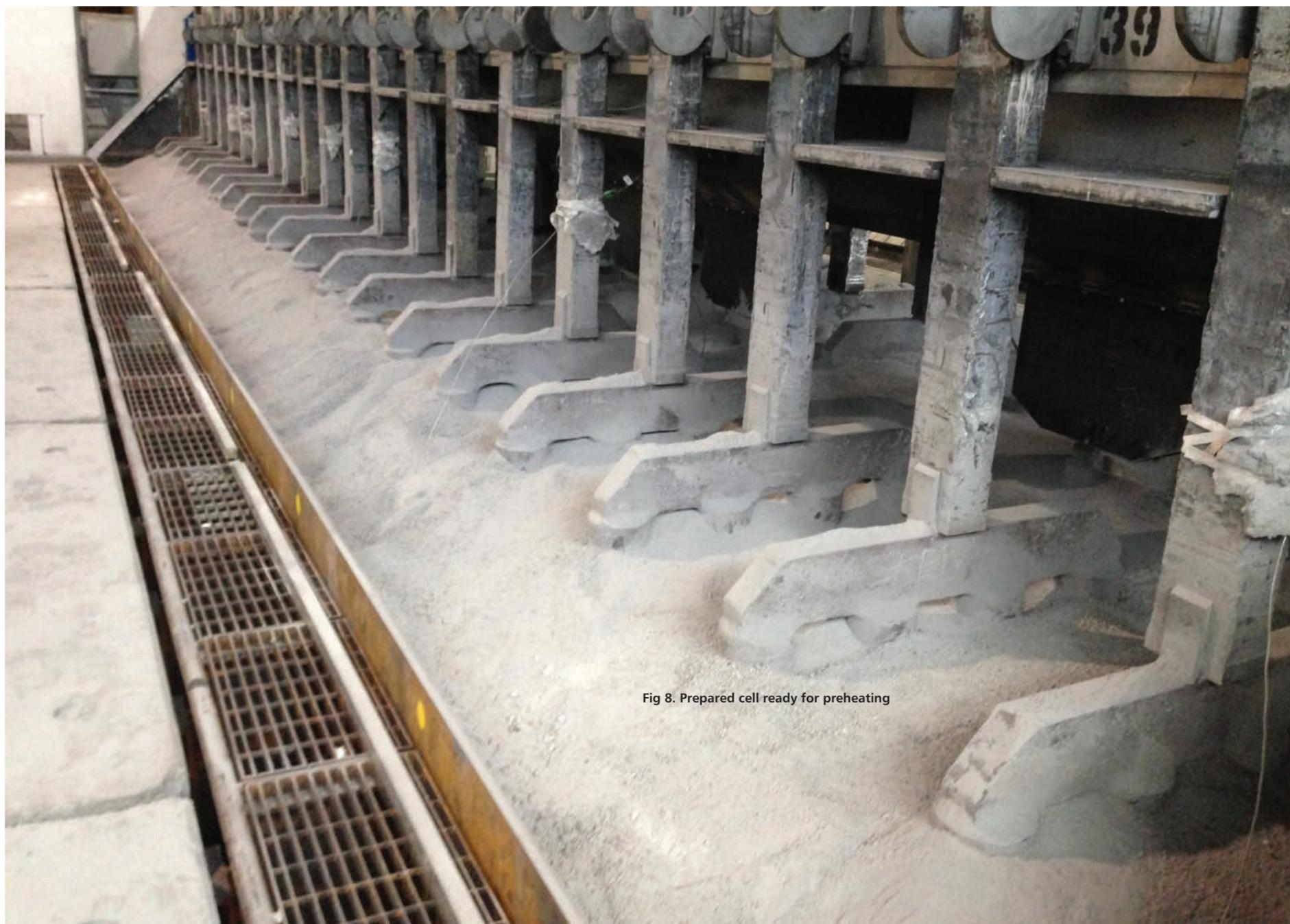
Fig 8. Prepared cell ready for preheating
