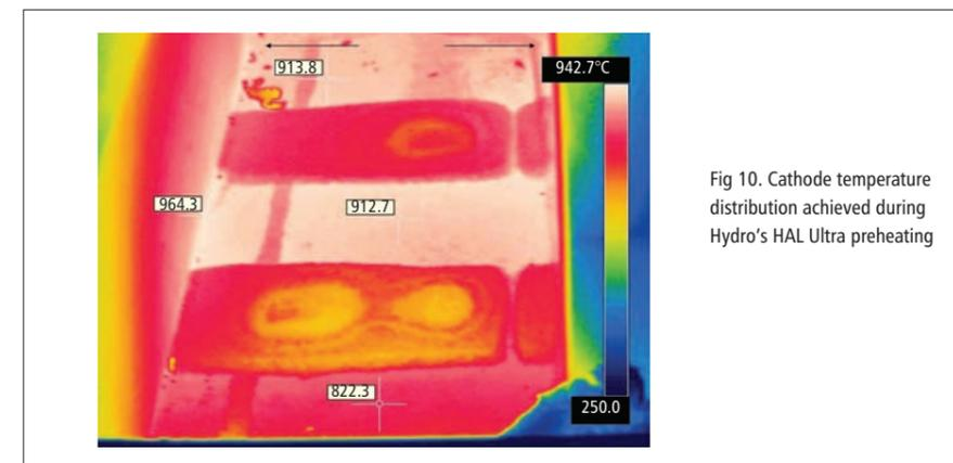
Fig 10. Cathode temperature distribution achieved during Hydro's HAL Ultra preheating
