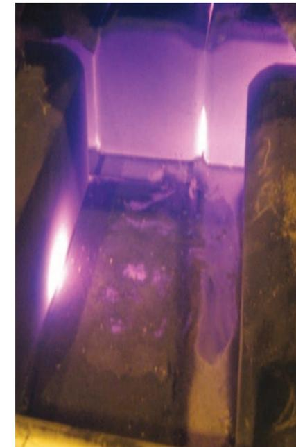
Fig 2. Example of a hot spot developing under an anode during preheating
