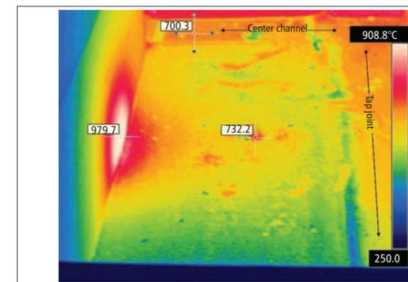
Fig 3. Thermogram of the same area of Figure 2 showing the temperature variations of the surface
