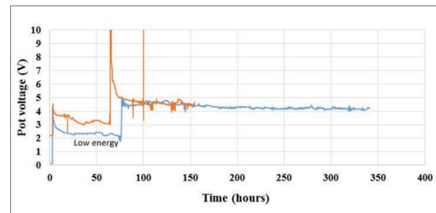
Fig 11. Cell voltage evolution during preheating and the first few days of early life for traditional and low energy strategies
