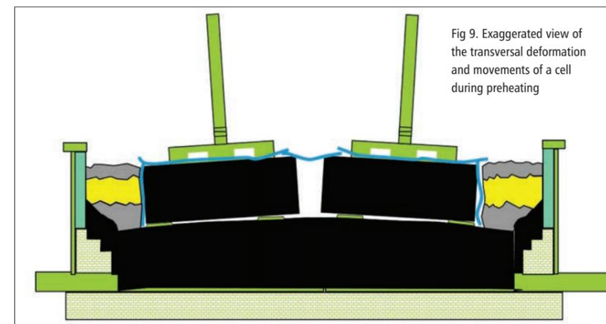
Fig 9. Exaggerated view of the transversal deformation and movements of a cell during preheating
