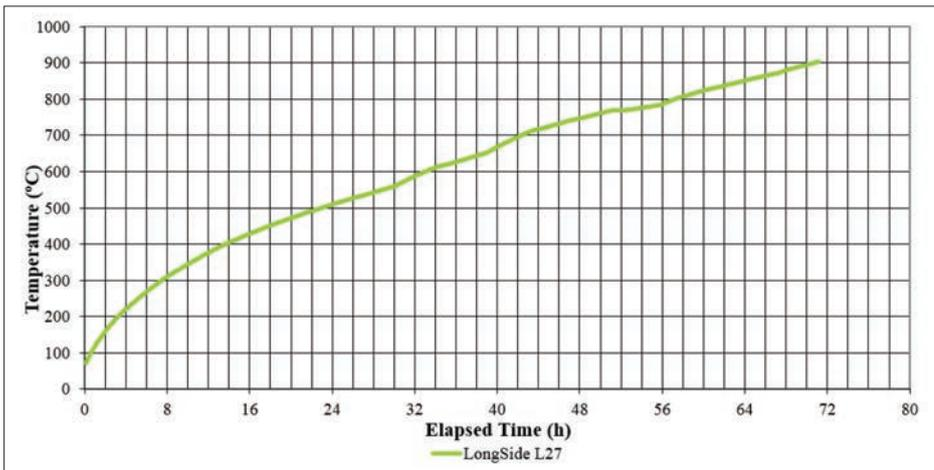
Fig 12. Example of long side temperature evolution during HAL Ultra preheat
