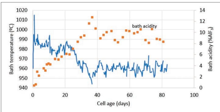
Fig 13. Bath temperature and acidity during early life and beyond for a low energy cell
