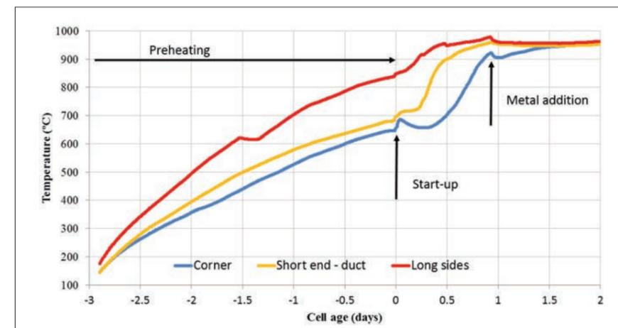
Fig 4. Temperature evolution at the top edge of cathode blocks during preheating and start-up
