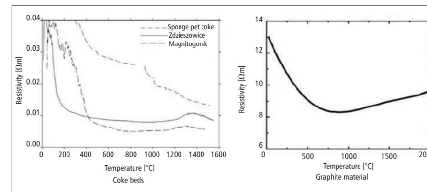
Fig 6. Resistivity of coke beds (left) and of graphite (right) as a function of temperature
