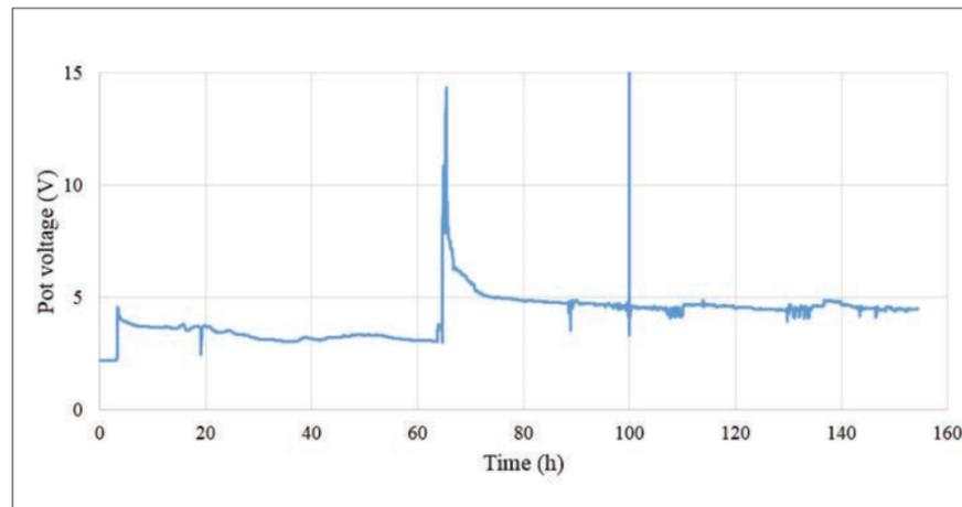
Fig 1. "Traditional" cell preheat and start-up voltage curve
